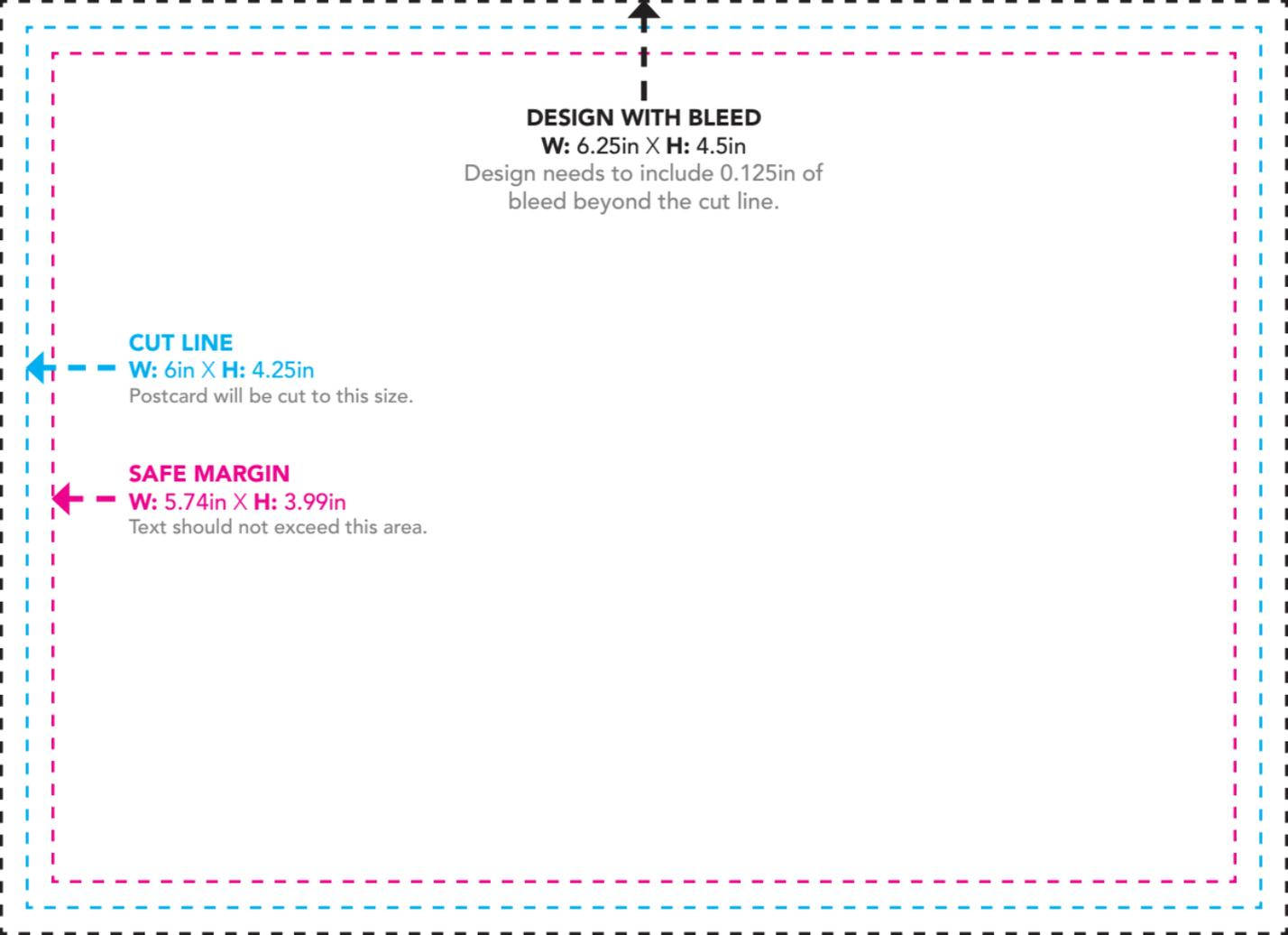
The diagram shows a rectangular layout for a postcard. It features three nested dashed lines: an outermost cyan line representing the bleed area, a middle magenta line representing the cut line, and an innermost magenta line representing the safe margin. A black dashed arrow points upwards from the top center of the design area towards the top edge of the bleed area.
